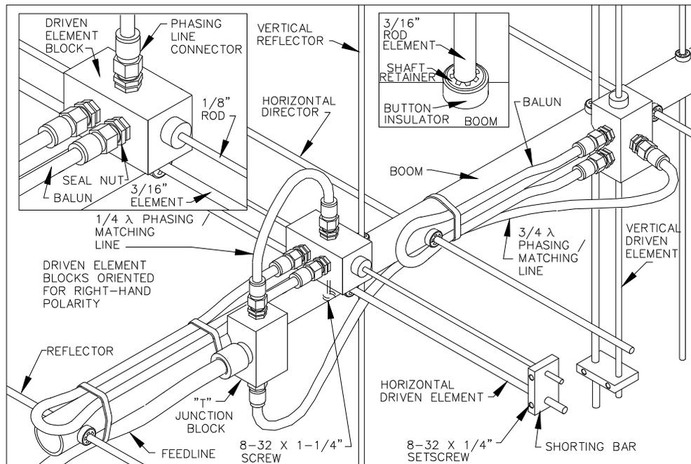
the block with the two balun connectors facing to rear.
