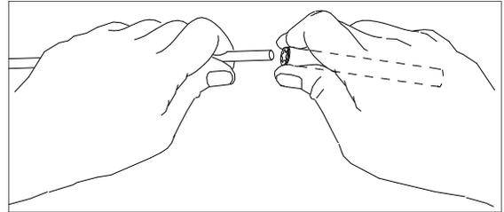
To install the stainless steel SHAFT RETAINERS, use thumb and forefinger to hold the retainer over the end of the PUSH TUBE ( 3/8" x 3" tube, supplied in the kit), internal fingers on retainer dished into tube. **HOLD THE ELEMENT FIRMLY TO PREVENT IT FROM SLIDING OFF CENTER** and press the retainer onto the
