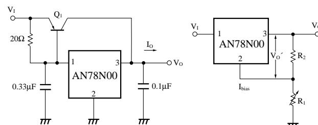
$$|V_O| = V_O' + \left( I_{bias} + \frac{V_O'}{R_2} \right) R_1$$
