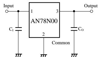
C<sub>i</sub> : is set when the input line is long.
