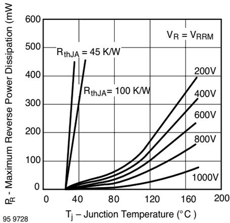
Figure 1. Max. Reverse Power Dissipation vs. Junction Temperature
