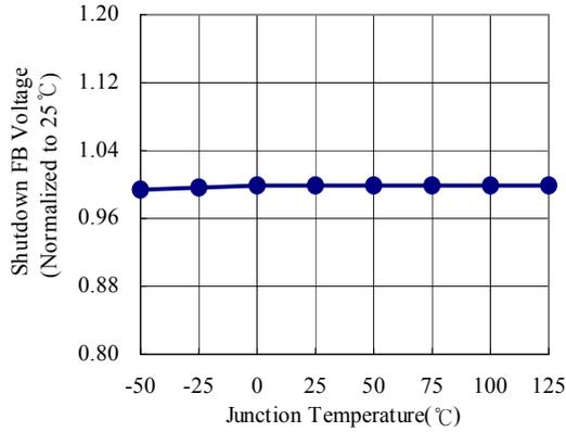
ShutDown Feedback Voltage vs. Temp
