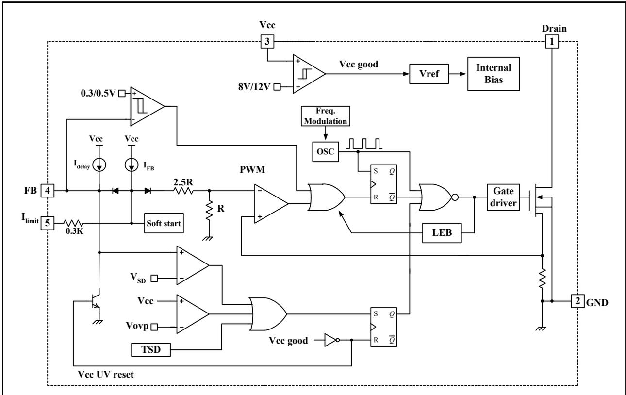
Figure 2. Functional Block Diagram of FSCM0765R
