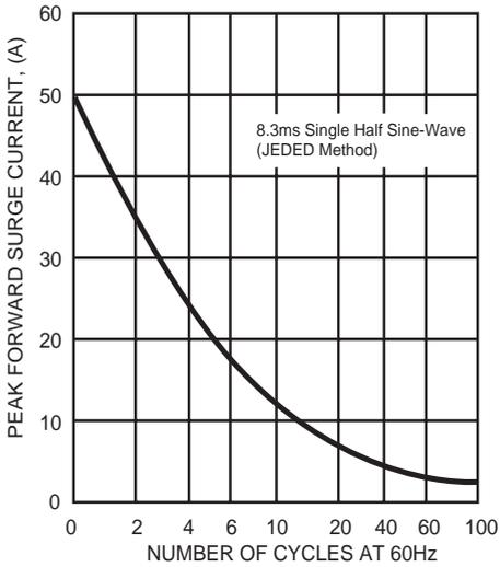
FIG. 2 - TYPICAL FORWARD CURRENT DERATING CURVE
