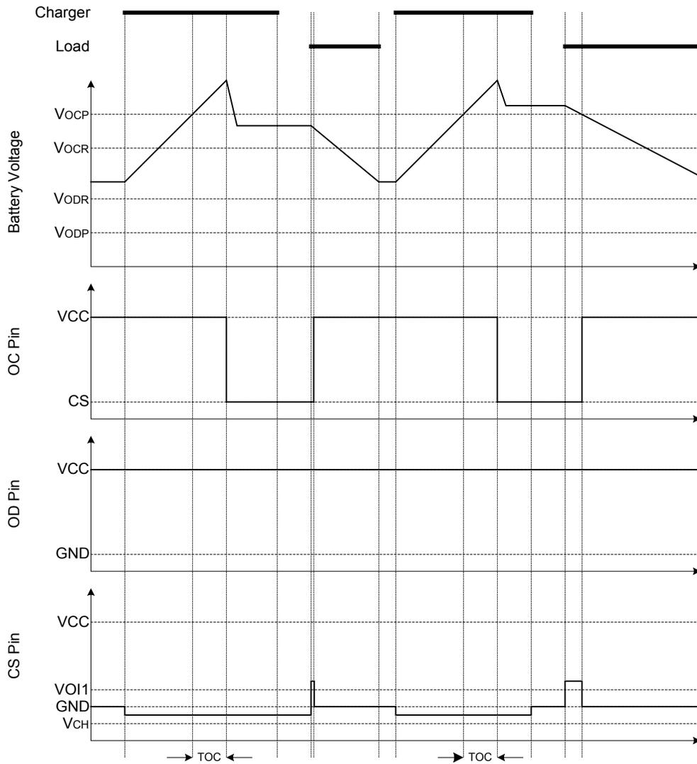
**2. Overdischarge Condition → Charging by a Charger → Normal Condition**
