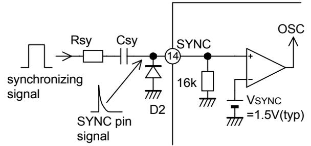
Fig.2 SYNC pin circuit (1)
