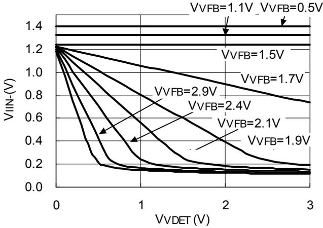
IDET pin voltage( $V_{IDET}$ ) vs. IIN- pin voltage( $V_{IIN-}$ )
