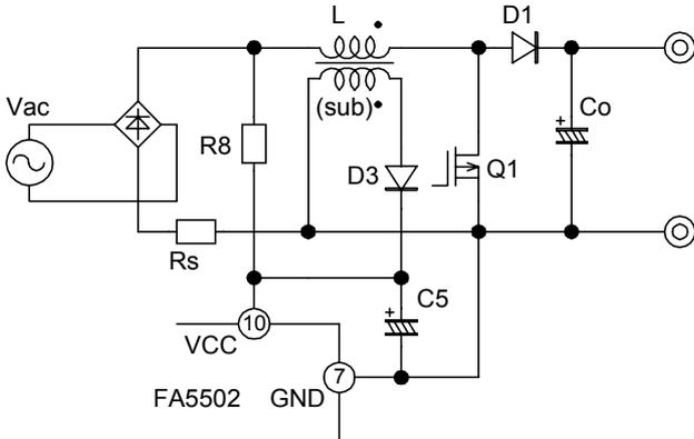
Fig.15 Vcc circuit (1)
