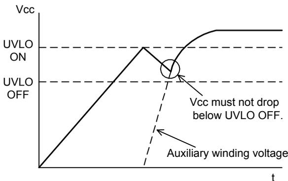
Fig.16 Vcc voltage at start up
