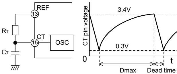
Fig.1 Oscillator circuit
