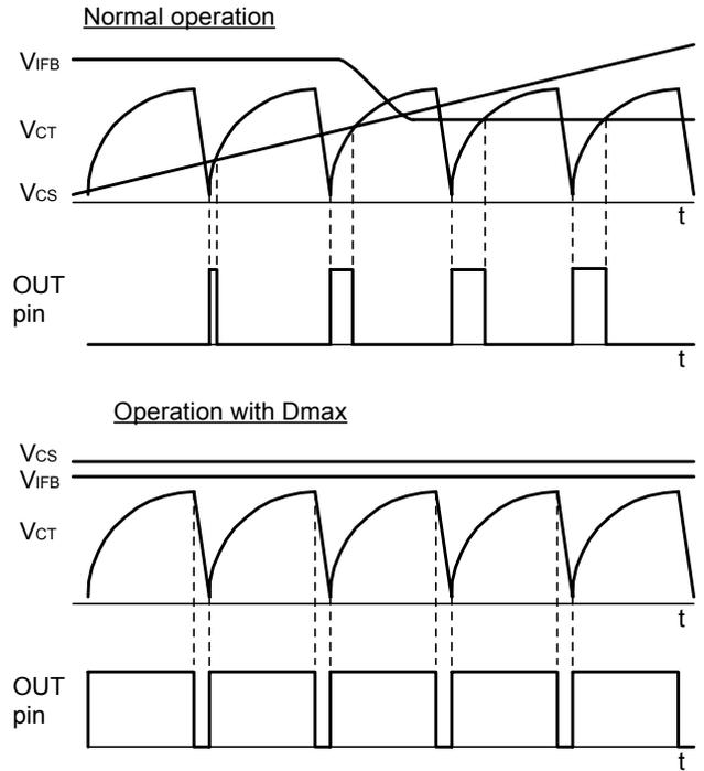
Fig.10 PWM comparator timing chart
