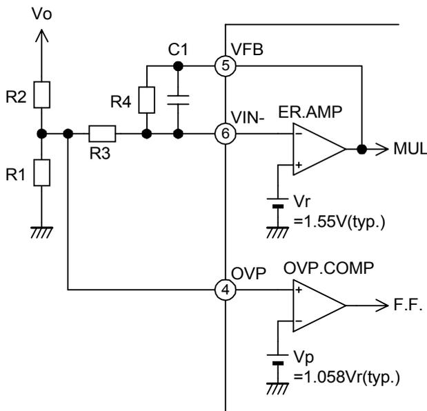
**Fig.6 Voltage error amplifier and overvoltage limiting circuit**
