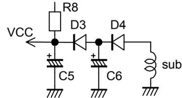
Fig.17 Vcc circuit (2)
