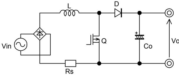
**Fig.19 Boost converter circuit**
