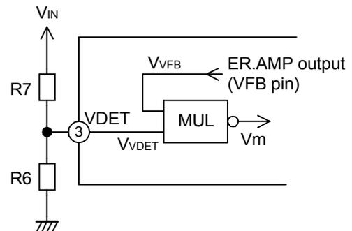
Fig.11 Multiplier circuit
