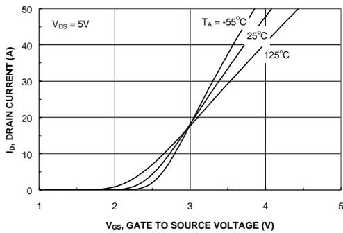
Figure 5. Transfer Characteristics.
