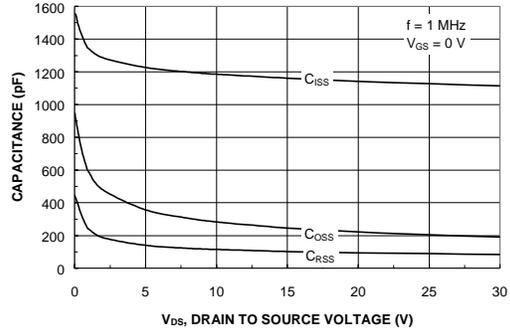
**Figure 8. Capacitance Characteristics.**
