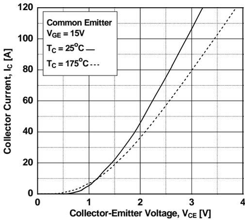
Figure 4. Transfer Characteristics
