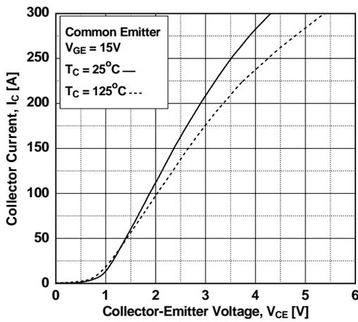
Figure 4. Transfer Characteristics
