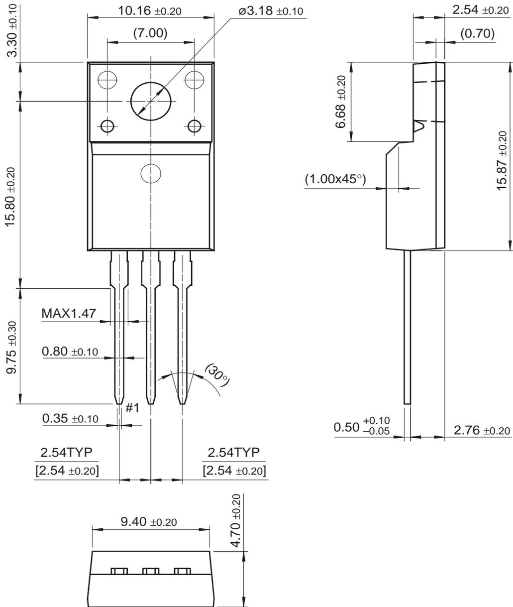
\* Front/Back Side Isolation Voltage : AC 2700V
