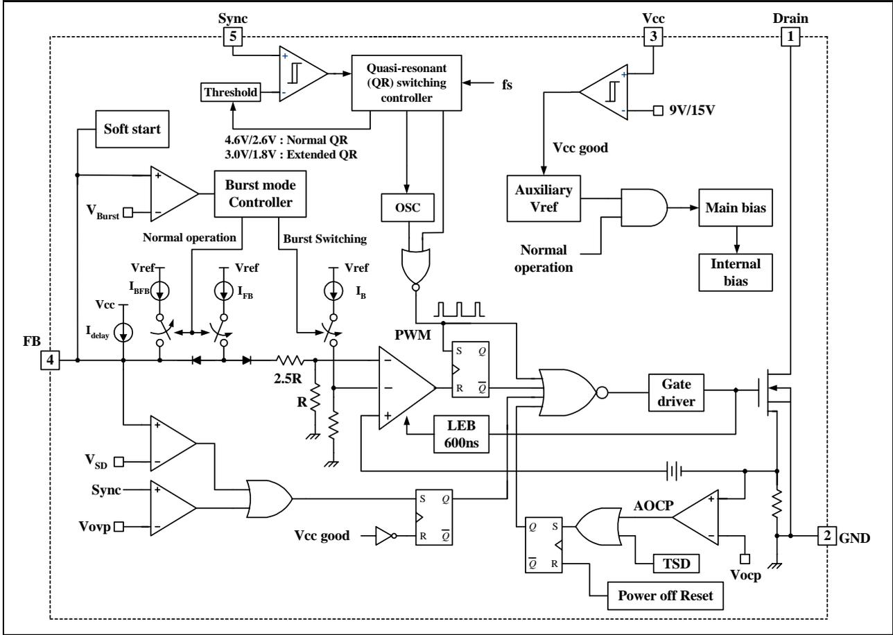
Figure 2. Functional Block Diagram of FSCQ0765RT
