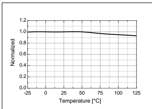
Figure 8. Initial Switching Frequency ( $f_S$ ) vs.  $T_A$
