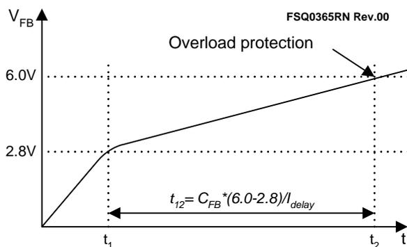
**Figure 24. Overload Protection**
