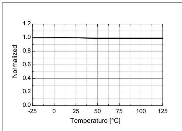
Figure 18. Shutdown Feedback Voltage ( $V_{SD}$ ) vs.  $T_A$
