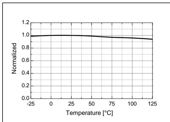
Figure 7. Start-up Charging Current ( $I_{CH}$ ) vs.  $T_A$
