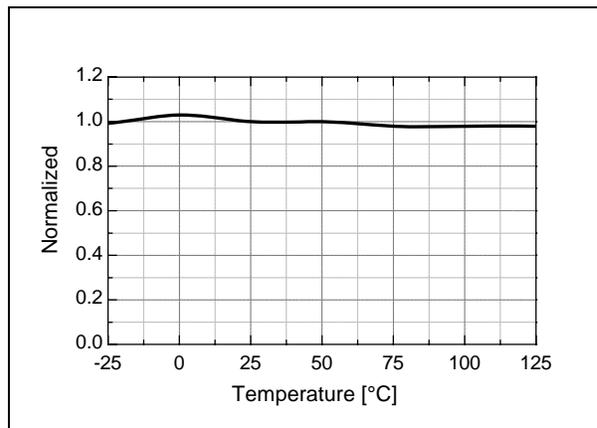
Figure 17. Sync Low Threshold Voltage ( $V_{SL}$ ) vs.  $T_A$
