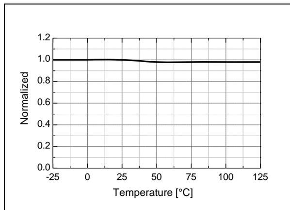
Figure 13. Burst-Mode High Threshold Voltage ( $V_{burh}$ ) vs.  $T_A$
