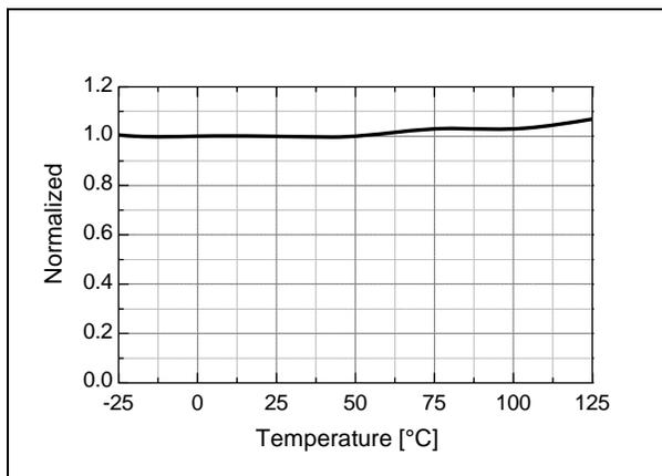
Figure 10. Blanking Time ( $t_B$ ) vs.  $T_A$
