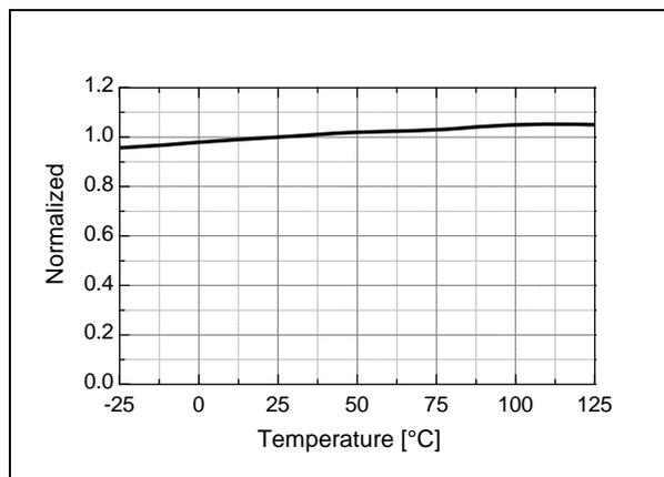
Figure 15. Peak Current Limit ( $I_{LIM}$ ) vs.  $T_A$
