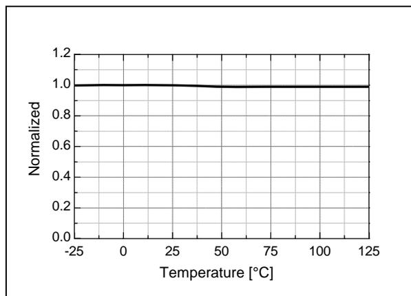
Figure 19. Over-Voltage Protection ( $V_{OP}$ ) vs.  $T_A$
