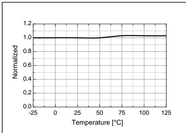
Figure 16. Sync High Threshold Voltage ( $V_{SH}$ ) vs.  $T_A$
