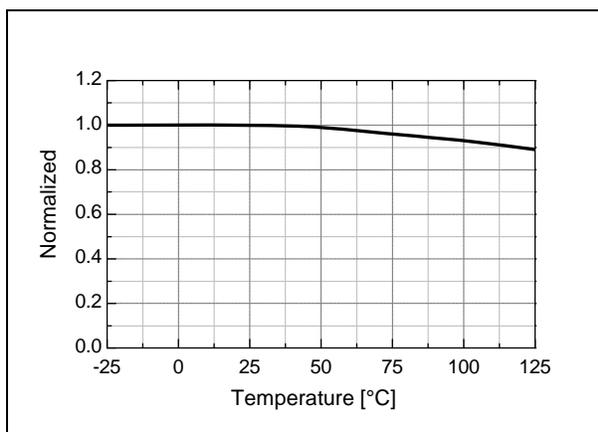
Figure 12. Shutdown Delay Current ( $I_{DELAY}$ ) vs.  $T_A$
