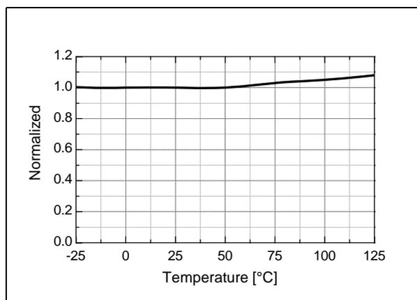
Figure 9. Maximum On Time ( $t_{ON.MAX}$ ) vs.  $T_A$
