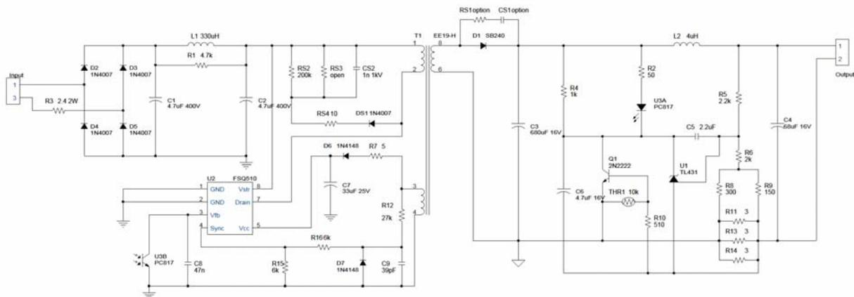
Figure 13. FSQ510 Schematic
