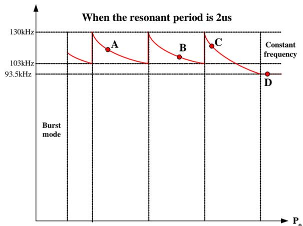
Figure 12. Switching Frequency Range of the Advanced QRC
