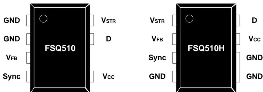
Figure 3. Package diagrams for FSQ510 and FSQ510H
