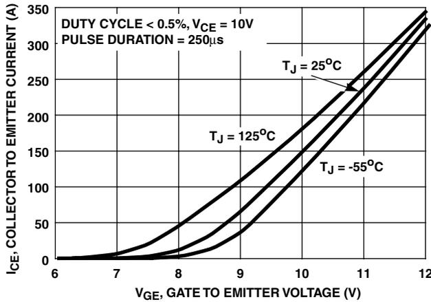
FIGURE 13. TRANSFER CHARACTERISTIC
