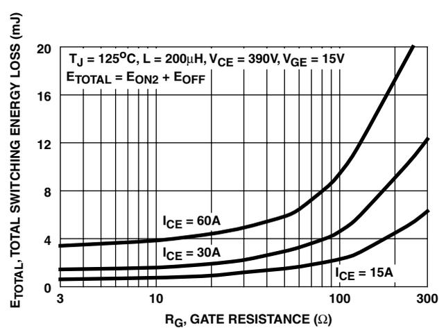
FIGURE 16. TOTAL SWITCHING LOSS vs GATE RESISTANCE
