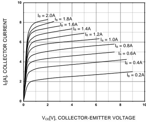
Figure 1. Static Characteristic
