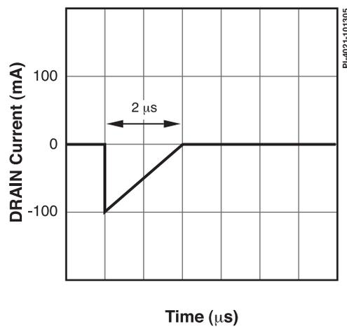
Figure 11. Peak Negative Pulsed DRAIN Current Waveform.
