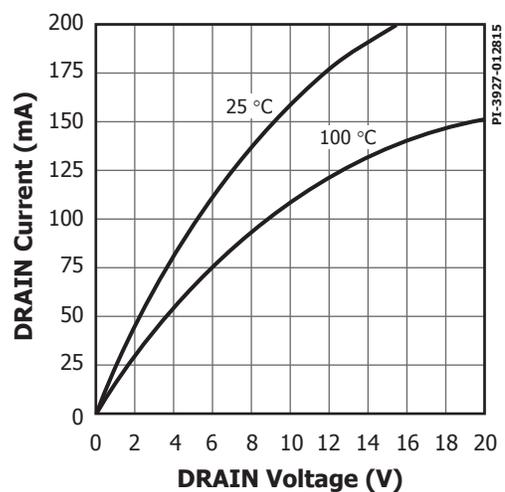
Figure 17. Output Characteristics.
