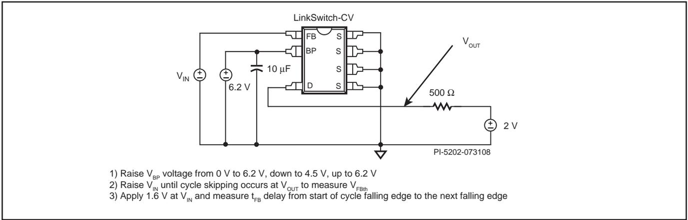
Figure 19. Test Set-up for Feedback Pin Measurements.
