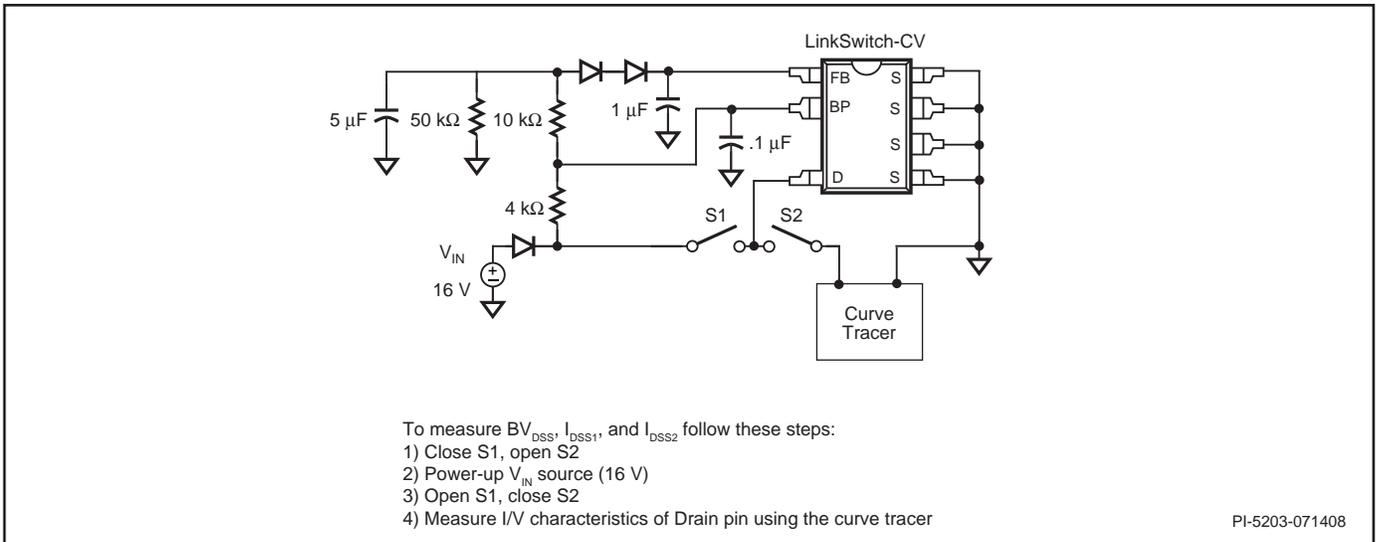
Figure 20. Test Set-up for Leakage and Breakdown Tests.
