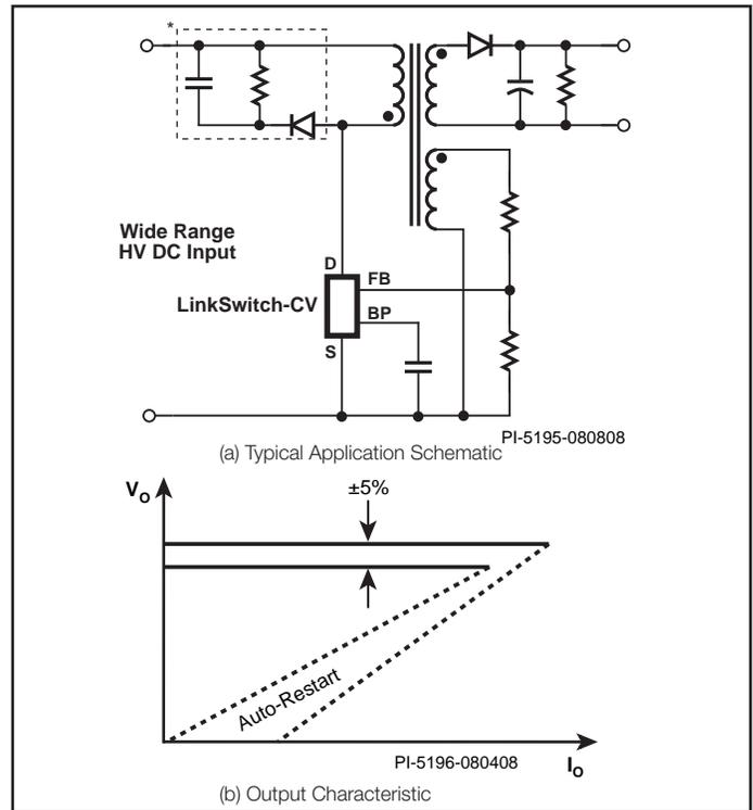
Figure 1. Typical Application Schematic (a) and Output Characteristic Envelope (b).
