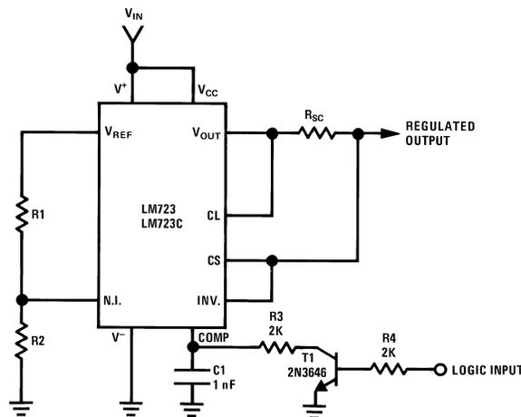
**Note:** Current limit transistor may be used for shutdown if current limiting is not required.
