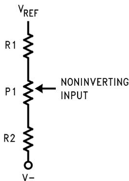
Figure 28. Output Voltage Adjust <sup>(1)</sup>
