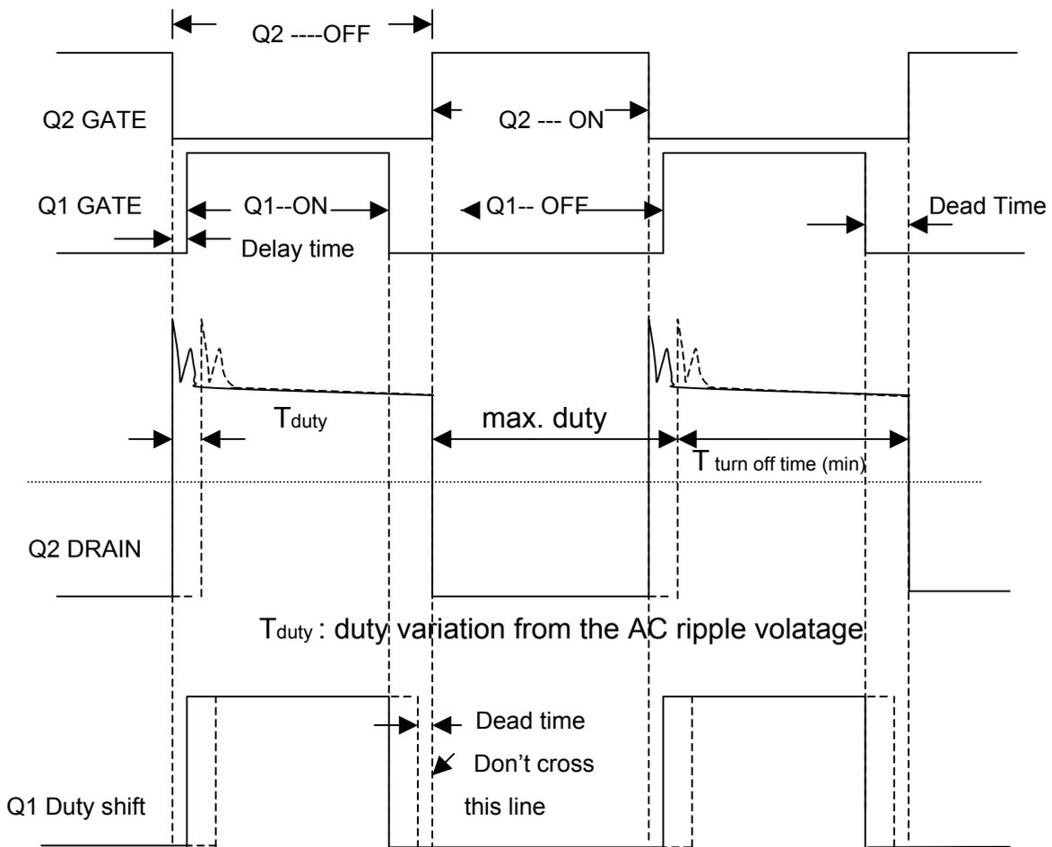
**b. Synchronous signal from primary side**
