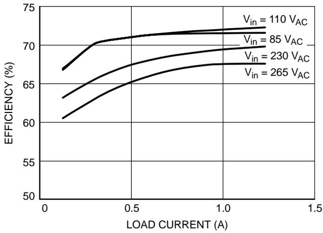
Figure 36. Converter Efficiency
