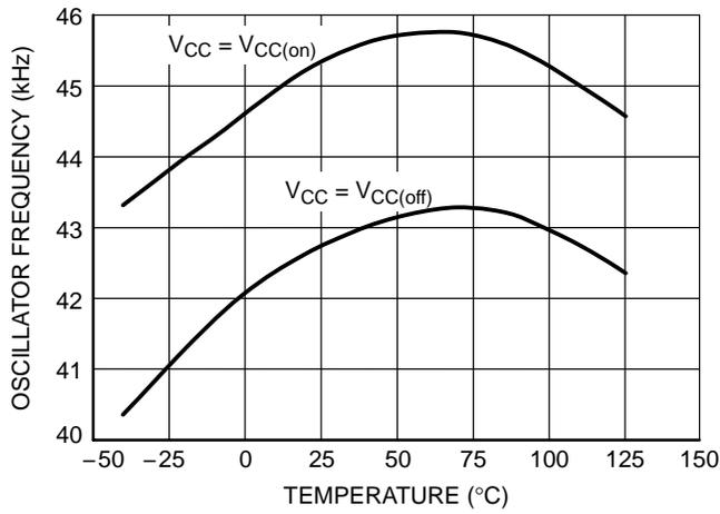
**Figure 5. Oscillator Frequency (A Suffix) versus Temperature**
