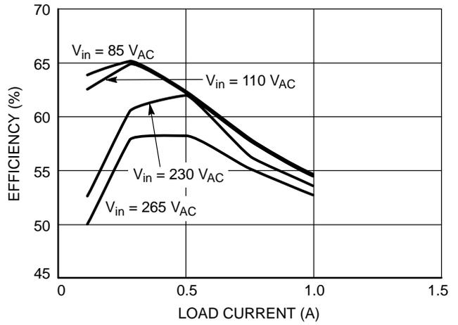
Figure 37. Charger Efficiency
