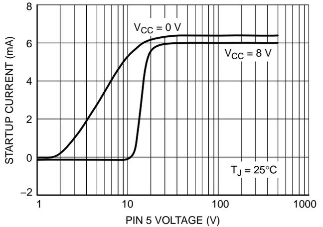
Figure 22. Startup Current versus Pin 5 Voltage
