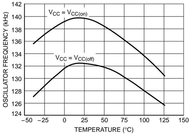
**Figure 7. Oscillator Frequency (C Suffix) versus Temperature**
