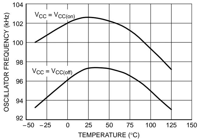
**Figure 6. Oscillator Frequency (B Suffix) versus Temperature**
