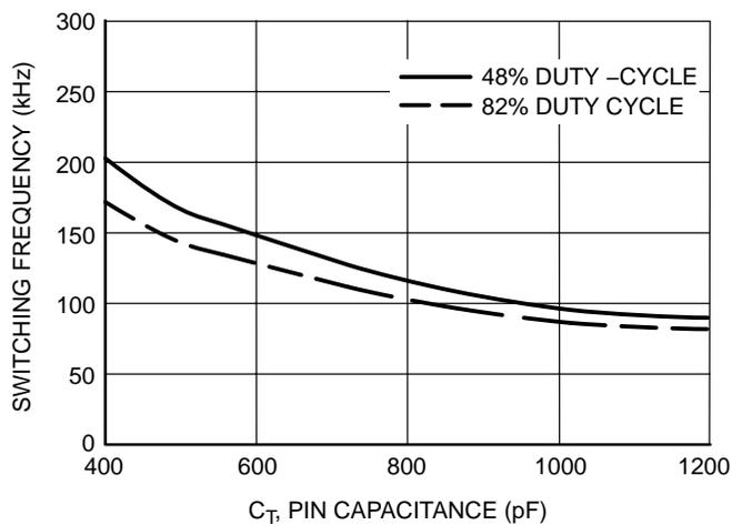
**Figure 31. Switch Frequency vs.  $C_T$  Pin Capacitance**
