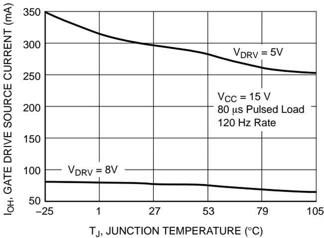
**Figure 13. Gate Drive Source Capability vs. Junction Temperature**
