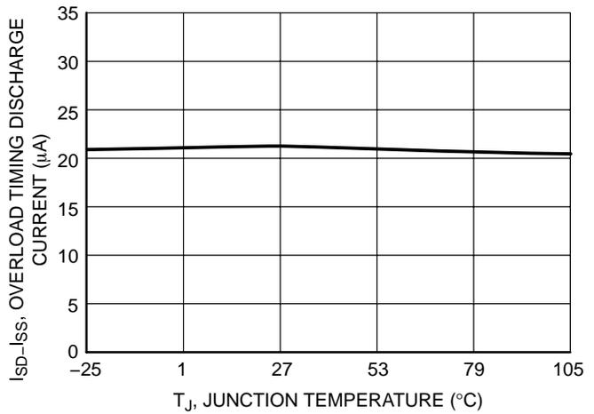
**Figure 10. Overload Timing Discharge Current vs. Junction Temperature**
