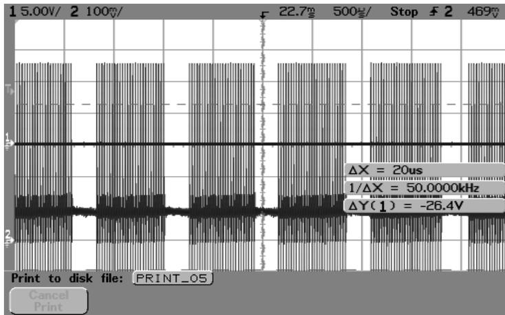
Figure 44. Skip Mode Switching Waveform at Light Load
