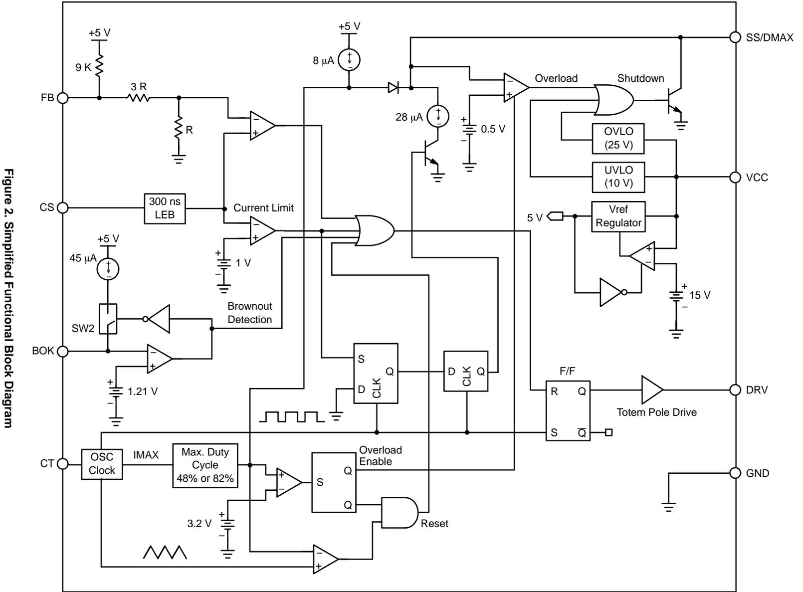
Figure 2. Simplified Functional Block Diagram
