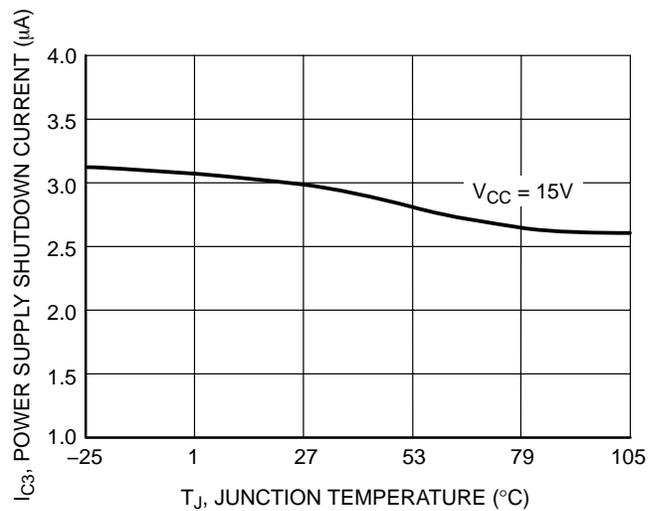
**Figure 26. Power Supply Shutdown Current vs. Junction Temperature**
