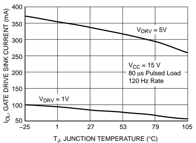
**Figure 14. Gate Drive Sink Capability vs. Junction Temperature**
