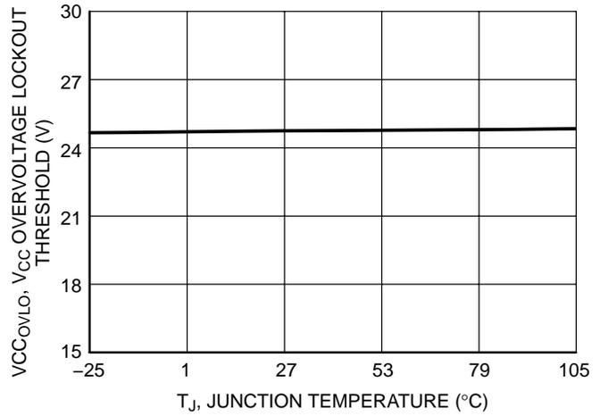
**Figure 22. V<sub>CC</sub> Overvoltage Lockout Threshold vs. Junction Temperature**
