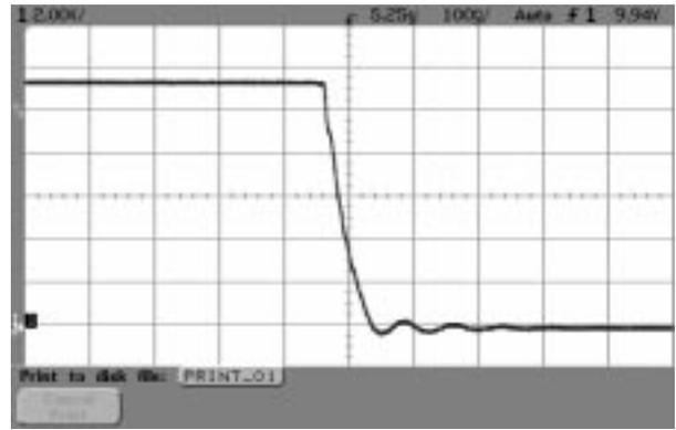
**Figure 28. Fall Time of Gate Drive Waveform**
