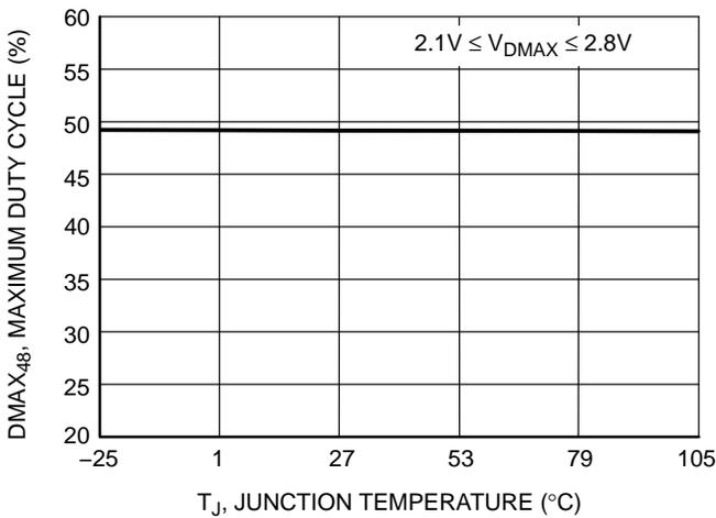
**Figure 19. Maximum Duty Cycle, DMAX<sub>48</sub> vs. Junction Temperature**
