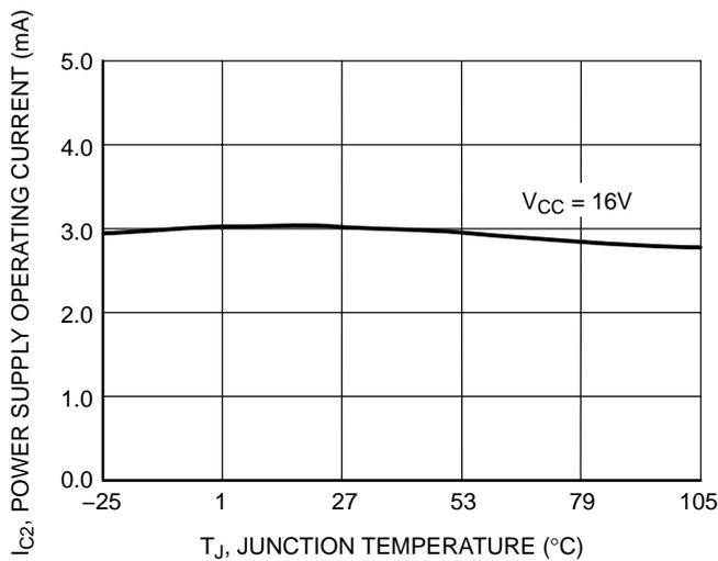
**Figure 25. Power Supply Operating Current vs. Junction Temperature**
