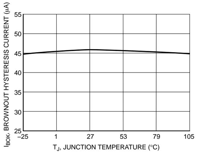
**Figure 18. Brownout Hysteresis Current vs. Junction Temperature**
