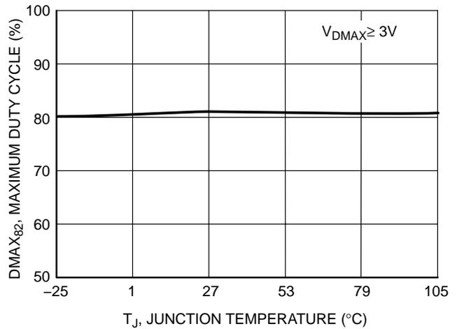
**Figure 20. Maximum Duty Cycle, DMAX<sub>82</sub> vs. Junction Temperature**
