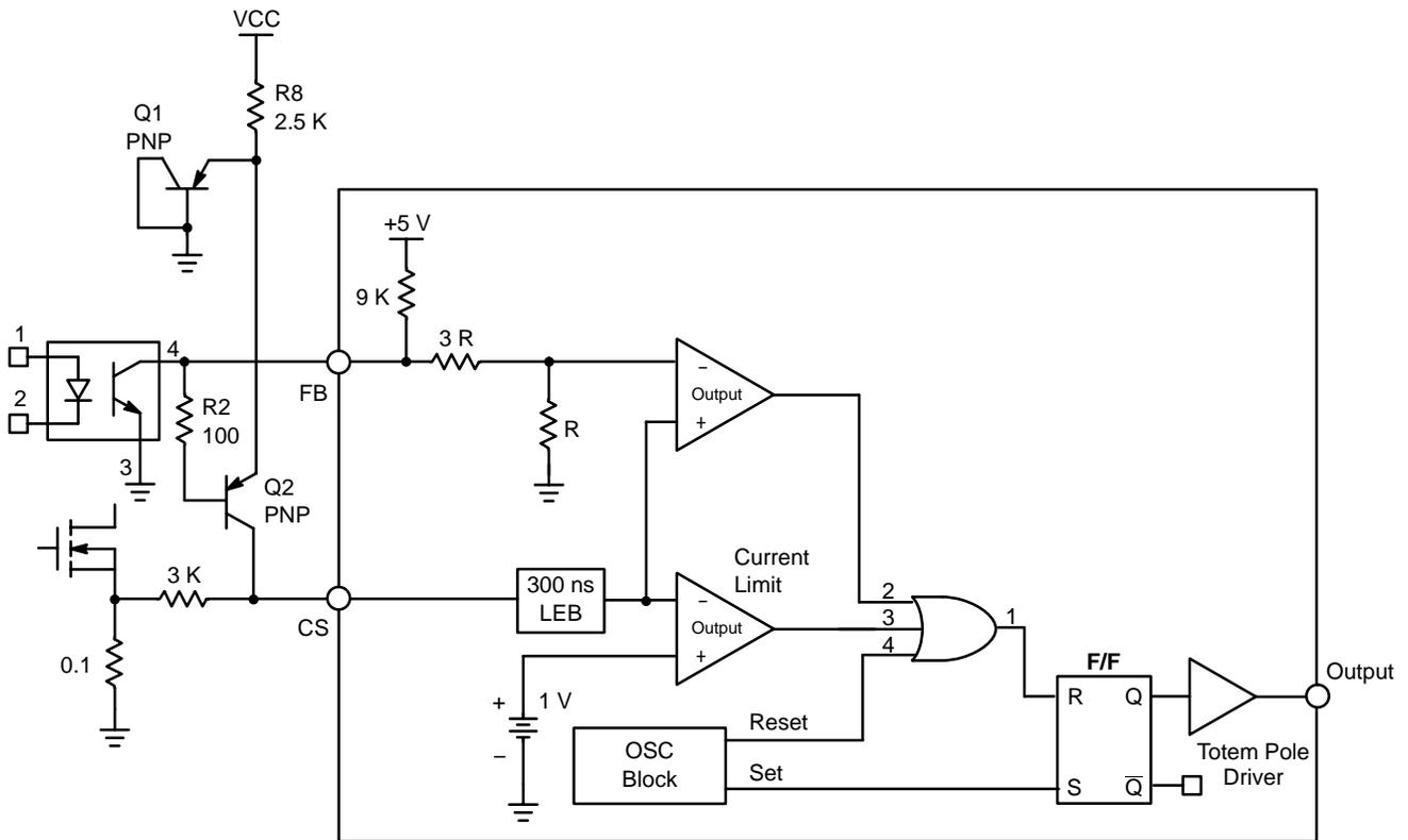
Figure 43. Suggested Solution for Better Light Load Regulation
