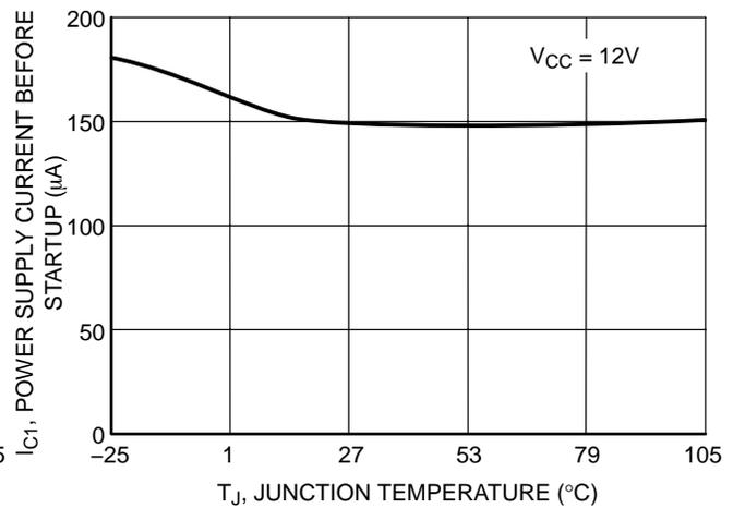
**Figure 24. Power Supply Current Startup vs. Junction Temperature**
