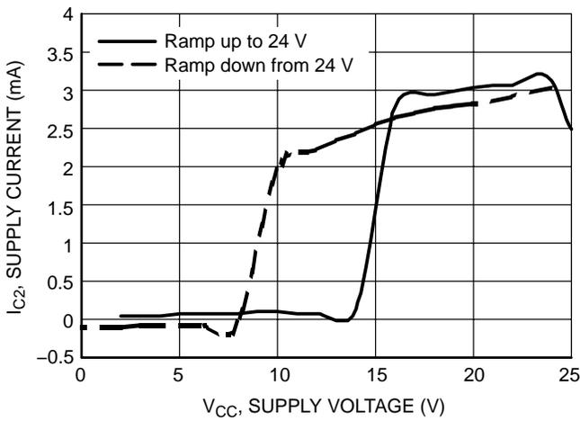
**Figure 29. Supply Current vs. Supply Voltage**
