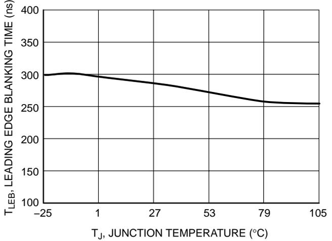
Figure 8. Leading Edge Blanking Time vs. Junction Temperature
