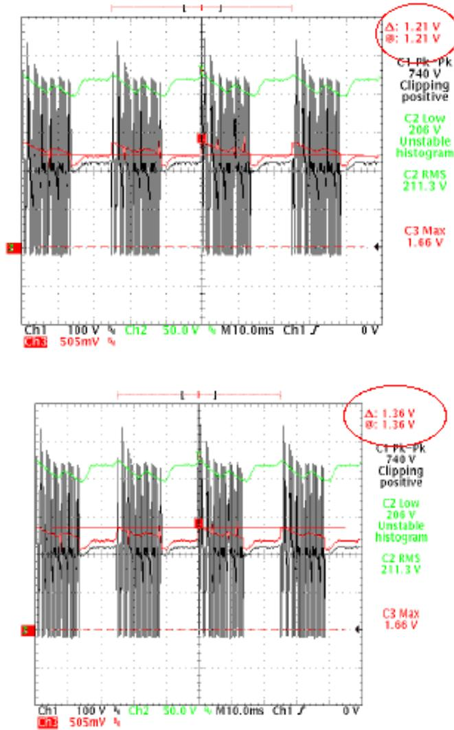
Channel 1: The MOSFET's  $V_{DS}$  Switching Waveform
