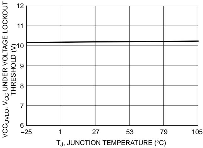
**Figure 21. V<sub>CC</sub> Under Voltage Lockout Threshold vs. Junction Temperature**
