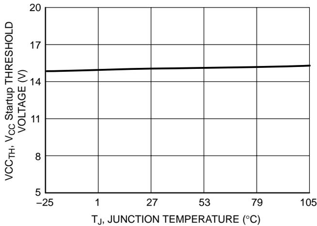
**Figure 23. V<sub>CC</sub> Startup Threshold Voltage vs. Junction Temperature**
