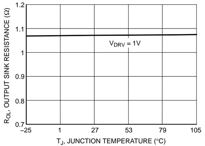
**Figure 12. Output Sink Resistance vs. Junction Temperature**
