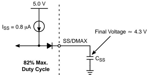
Figure 36. 82% Maximum Duty Cycle Selection
