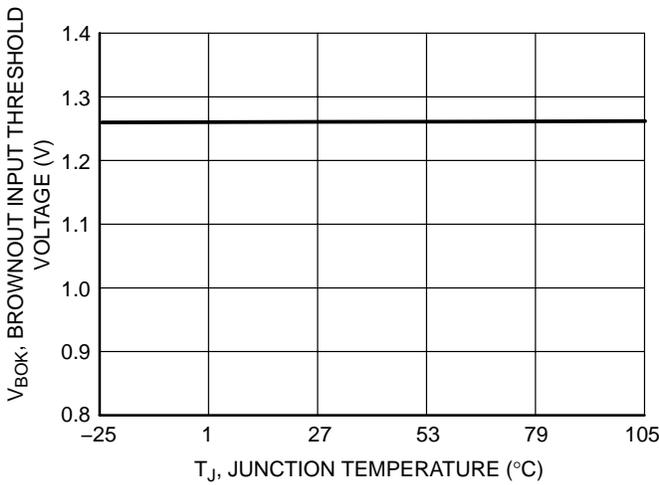
**Figure 17. Brownout Input Threshold Voltage vs. Junction Temperature**
