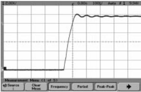
**Figure 27. Rise Time of Gate Drive Waveform**
