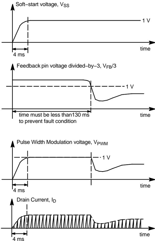
**Figure 29. Soft-Start (Time = 0 at  $V_{CC} = V_{CC(on)}$ )**
