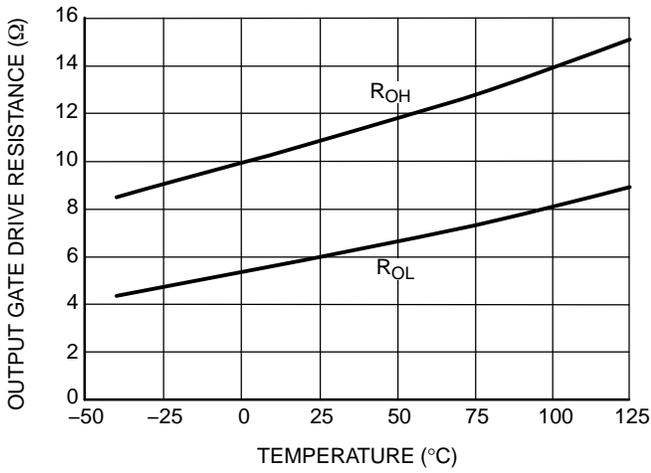
**Figure 5. Output Gate Drive Resistance vs. Temperature**
