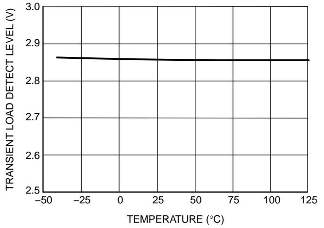
Figure 12. Transient Load Detection Level vs. Temperature
