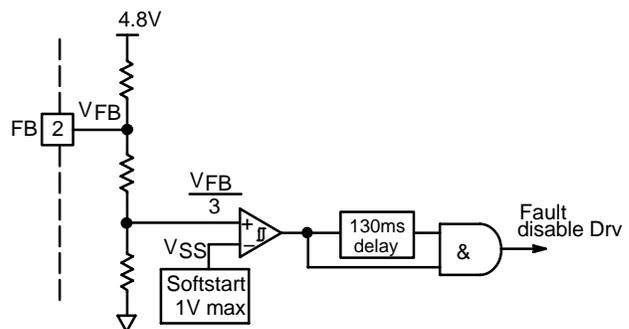
**Figure 35. Block Diagram of Timer-Based Fault Detection**
