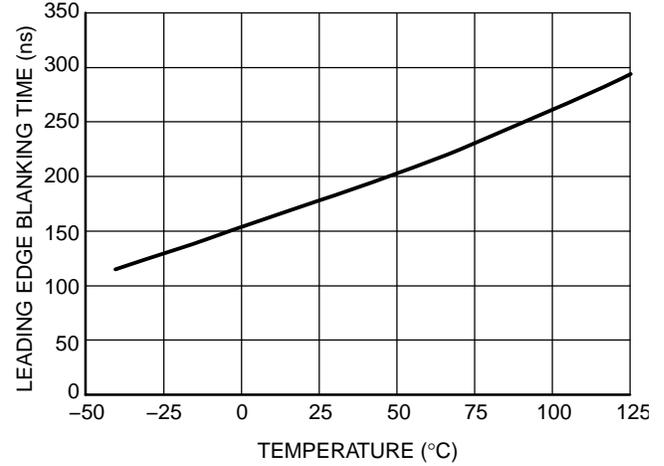
**Figure 8. Leading Edge Blanking Time vs. Temperature**
