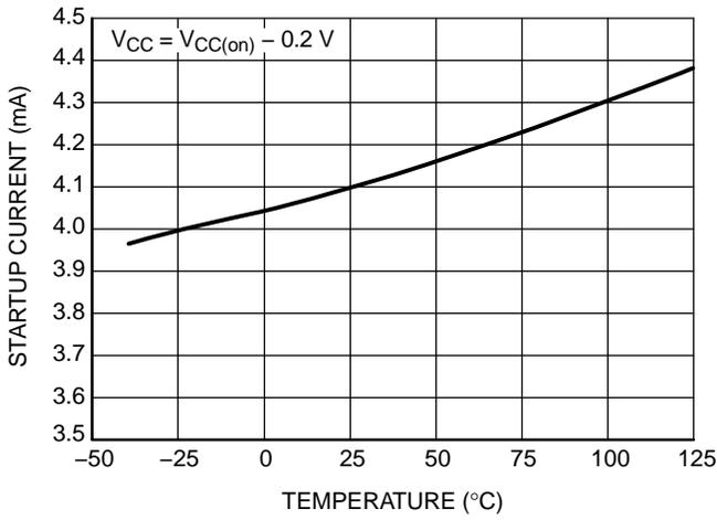
Figure 17. High Voltage Startup Current vs. Temperature
