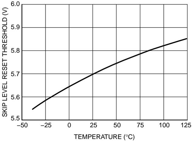
Figure 11. Skip Level Reset Threshold vs. Temperature
