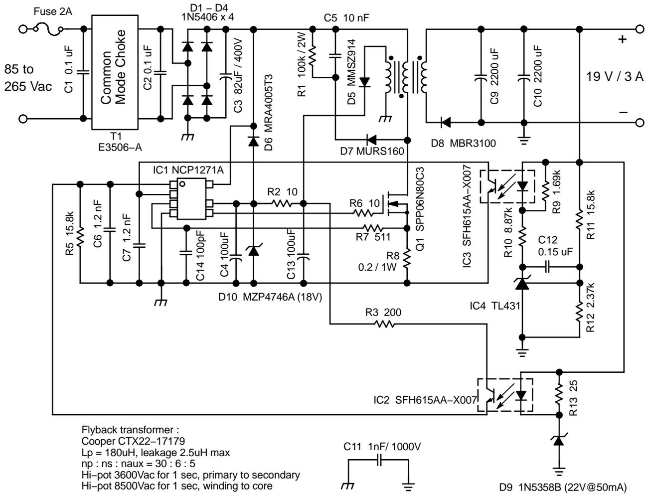
**Figure 42. 57 W Example Circuit Using NCP1271**
