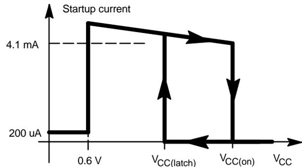
Figure 23. Startup Current at Various  $V_{CC}$  Levels
