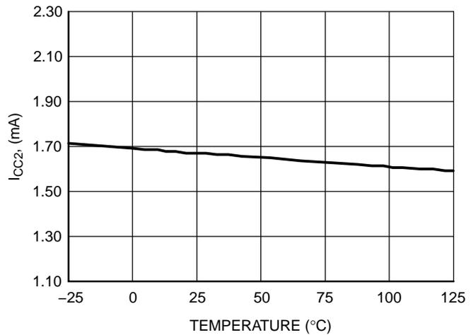
Figure 6. Current Consumption (1.0 nF Load) versus Temperature
