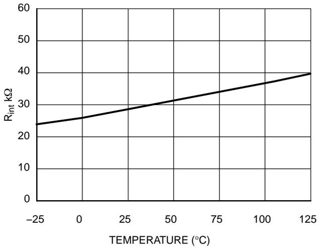
**Figure 15. DMG Pin Internal Resistance versus Temperature**
