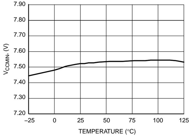
Figure 4. V<sub>CCMIN</sub> Threshold versus Temperature
