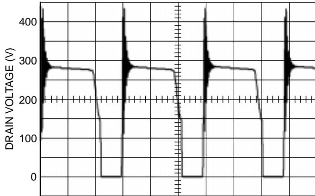
**Figure 23. The NCP1377 Operates in Borderline/Critical Operation**
