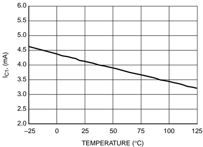
Figure 7. HV Current Source at V<sub>CC</sub> = 10 V versus temperature
