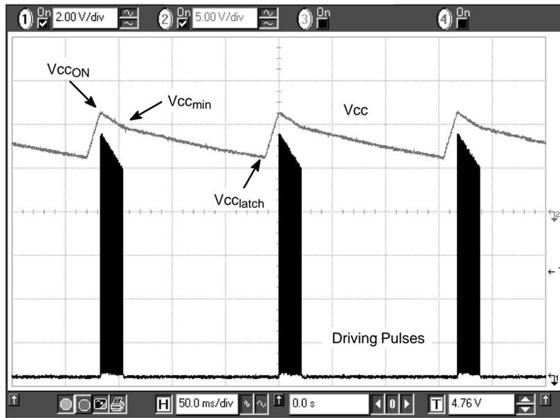
Figure 28. Typical Waveforms in Short Circuit Conditions
