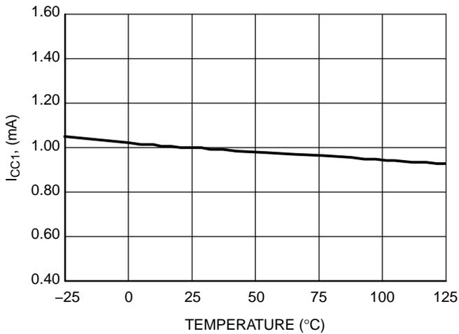
Figure 5. Current Consumption (No Load) versus Temperature
