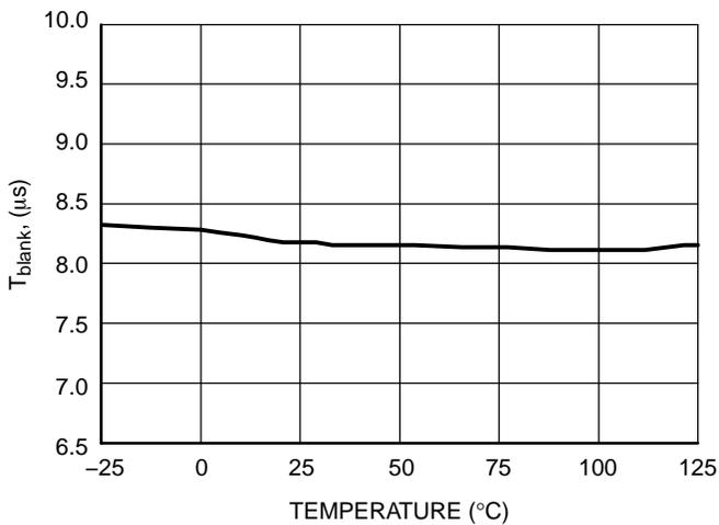
Figure 13. Minimum T<sub>OFF</sub> versus Temperature
