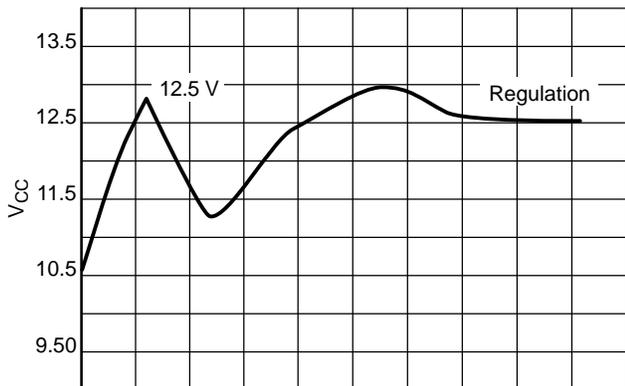
**Figure 17. A Typical Startup Sequence for the NCP1377**
