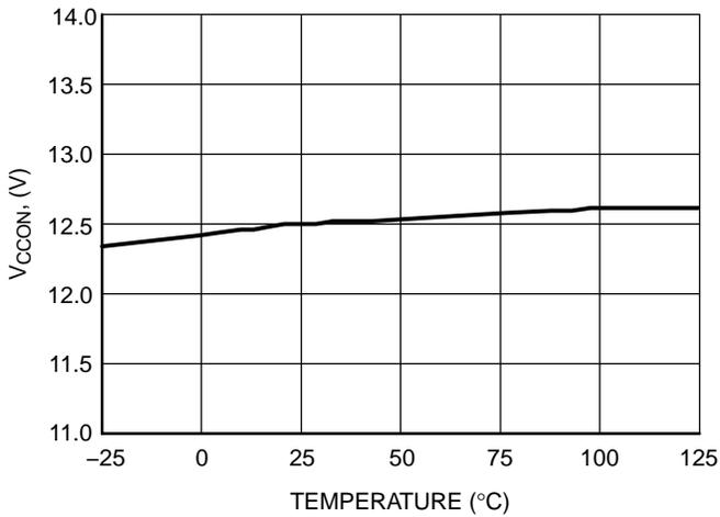
Figure 3. V<sub>CCON</sub> Threshold versus Temperature
