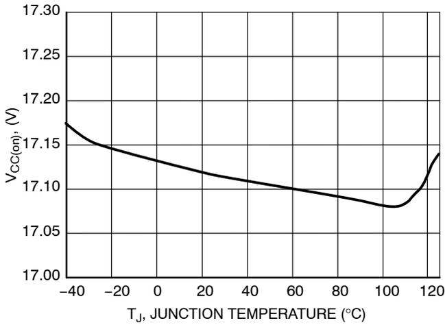
Figure 5. V<sub>CC(on)</sub> vs. Junction Temperature
