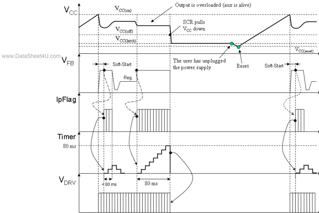
Figure 39. Latched Short-Circuit Protection on A and C Versions
