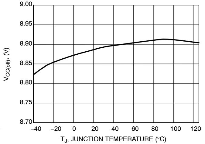
Figure 6. V<sub>CC(off)</sub> vs. Junction Temperature
