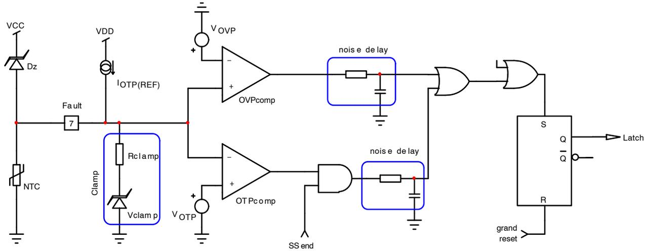
Figure 41. OVP/OTP Circuitry
