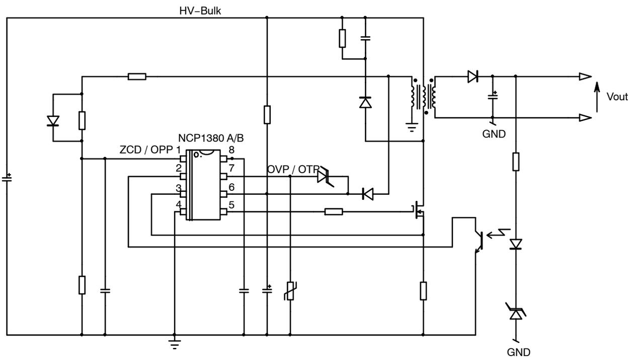
Figure 1. Typical Application Schematic for A and B Versions
