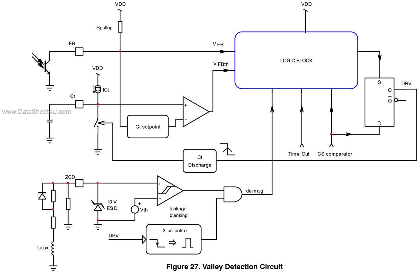
Figure 27. Valley Detection Circuit
