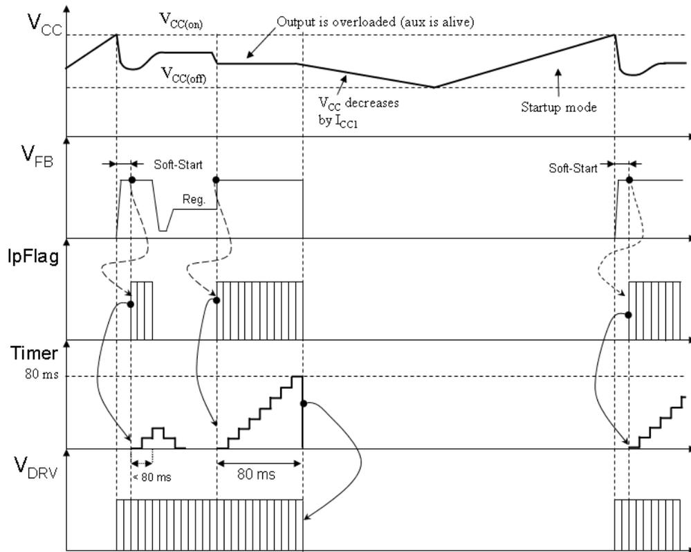
Figure 38. Auto-Recovery Short-Circuit Protection on B and D Versions
