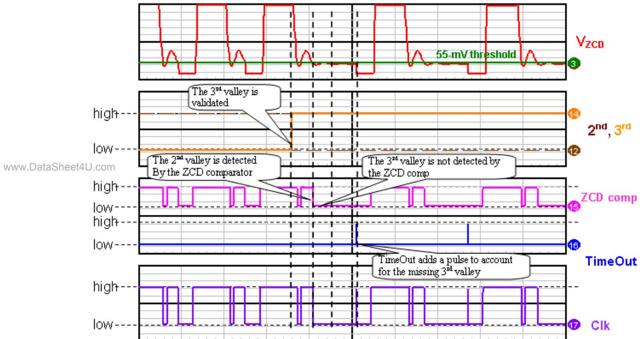
Figure 34. Time Out Case n°1: the 3<sup>rd</sup> Valley is Missing
