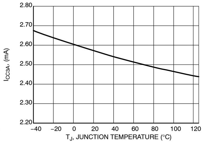
Figure 8. I<sub>CC3A</sub> vs. Junction Temperature
