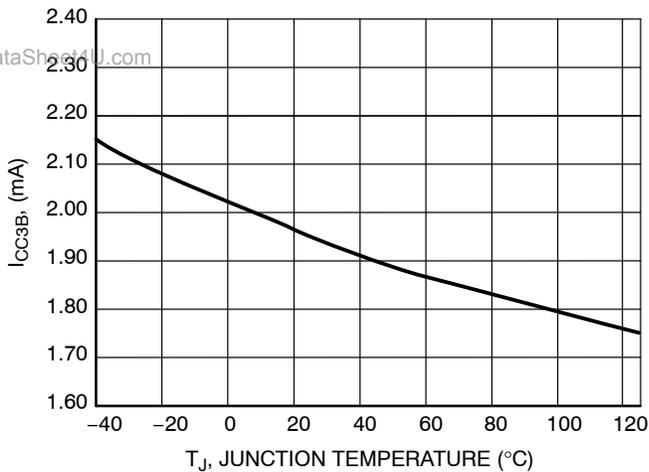
Figure 9. I<sub>CC3B</sub> vs. Junction Temperature
