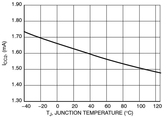
Figure 7. I<sub>CC2</sub> vs. Junction Temperature
