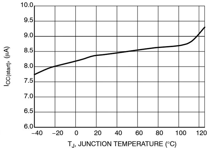
Figure 10. I<sub>CC(start)</sub> vs. Junction Temperature
