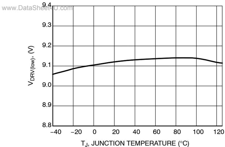
Figure 15.  $V_{DRV(low)}$  vs. Junction Temperature
