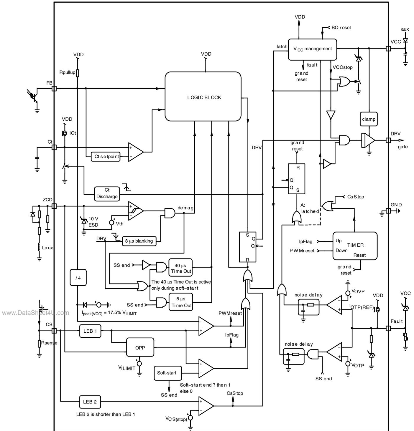
Figure 3. Internal Circuit Architecture for Versions A and B
