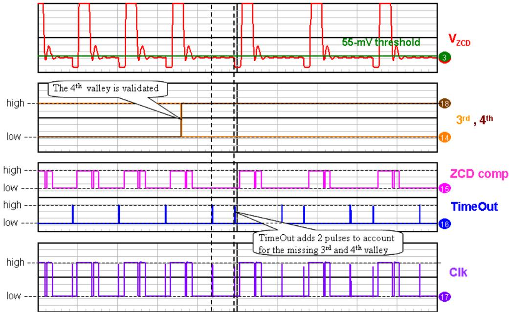
Figure 35. Time Out Case n°2: the 3<sup>rd</sup> and 4<sup>th</sup> Valley are Missing
