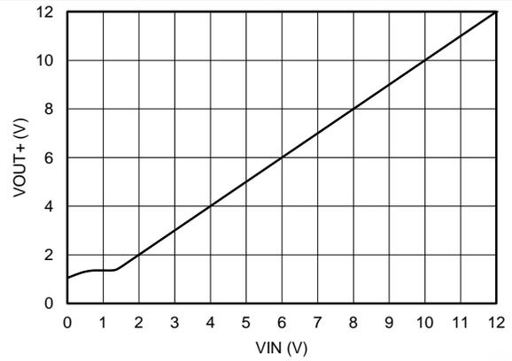
**Figure 6. Positive Output Voltage Node vs Input Voltage**
