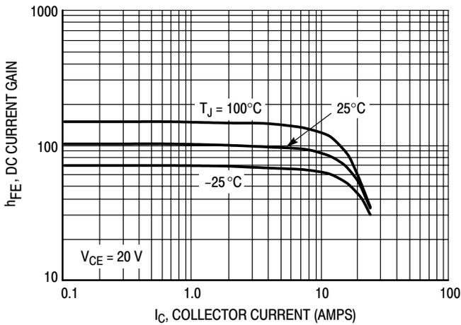
**Figure 3. DC Current Gain,  $V_{CE} = 20\text{ V}$**
