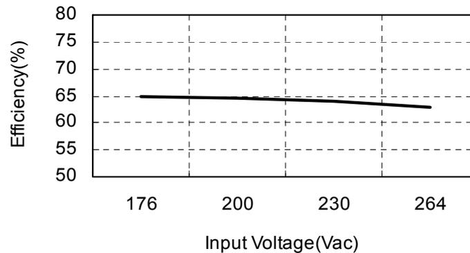
*Figure 2. Efficiency @200mA load*
