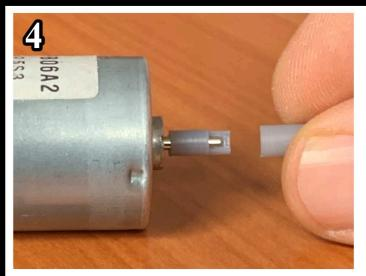
Remove the sleeve and insert the Worm Gear on the coupling.
