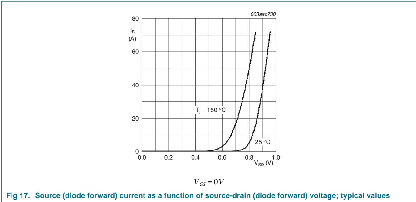
Fig 17. Source (diode forward) current as a function of source-drain (diode forward) voltage; typical values
