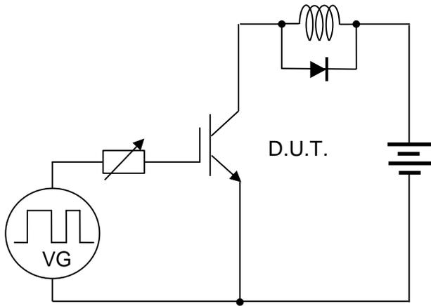
Fig.18 Inductive Load Circuit
