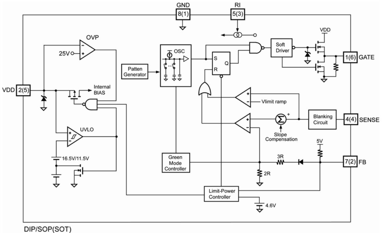
**Low Cost Green-Mode PWM Controller for Flyback Converters**
