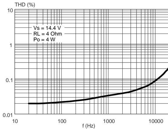
Figure 8. Distortion vs. Frequency (2W)
