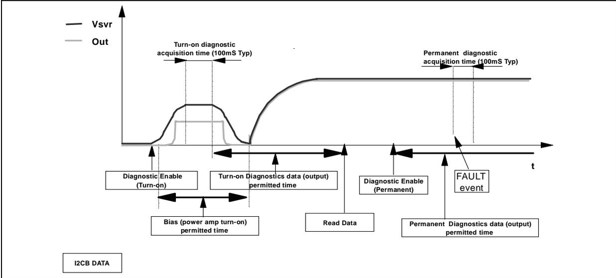
The information related to the outputs status is read and memorized at the end of the current pulse top. The acquisition time is 100 ms (typ.). No audible noise is generated in the process. As for SHORT TO GND /  $V_s$  the fault-detection thresholds remain unchanged from 26 dB to 12 dB gain setting. They are as follows:
