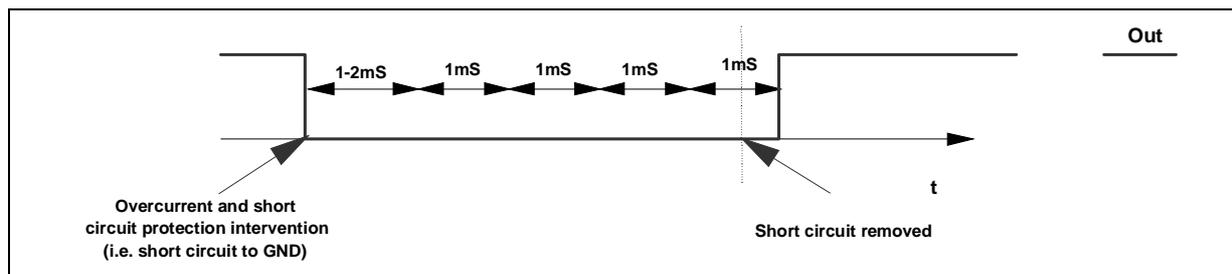
**Figure 18. Restart timing with Diagnostic Enable (Permanent)**
