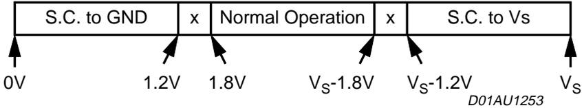
Concerning SHORT ACROSS THE SPEAKER / OPEN SPEAKER, the threshold varies from 26 dB to 12 dB gain setting, since different loads are expected (either normal speaker's impedance or high impedance). The values in case of 26 dB gain are as follows:
