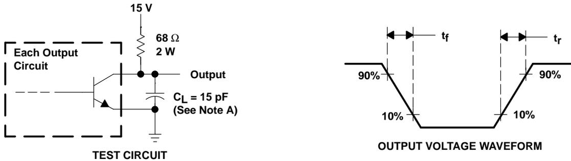
NOTE A.  $C_L$  includes probe and jig capacitance.
