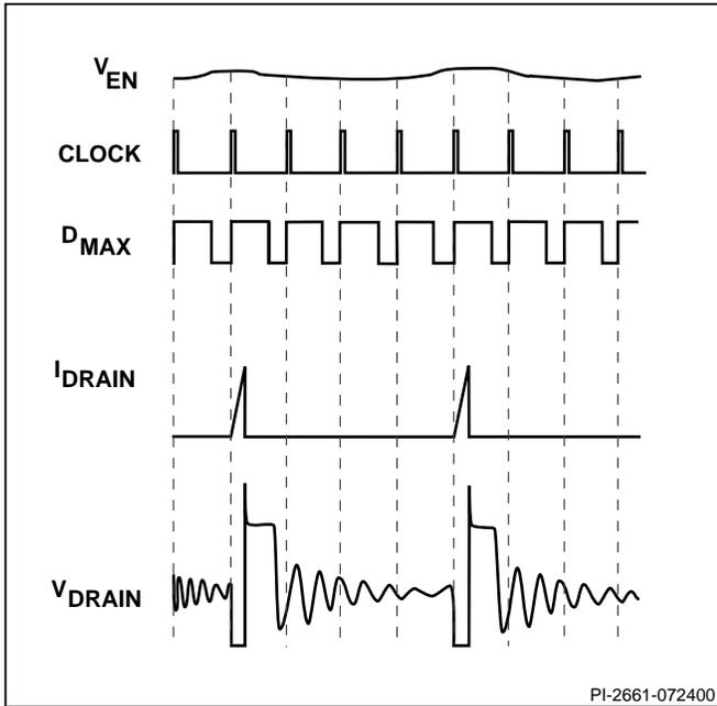
Figure 9. TinySwitch-II Operation at Very Light Load.
