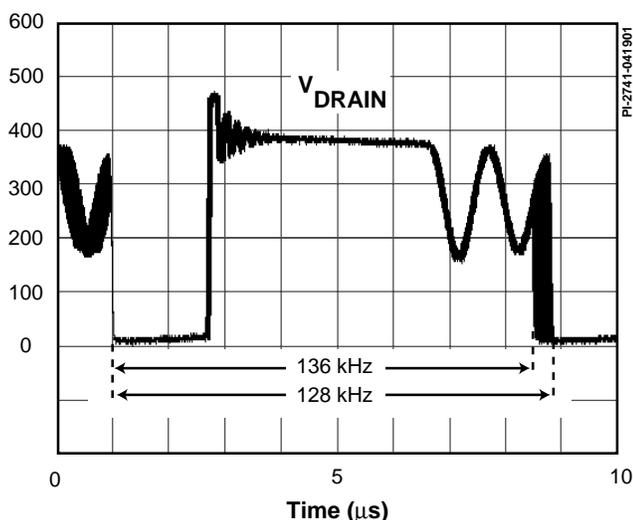
Figure 4. Frequency Jitter.
