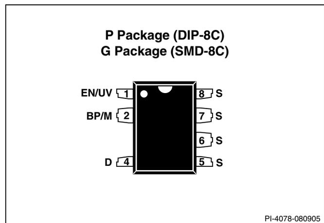
Figure 3. Pin Configuration.
