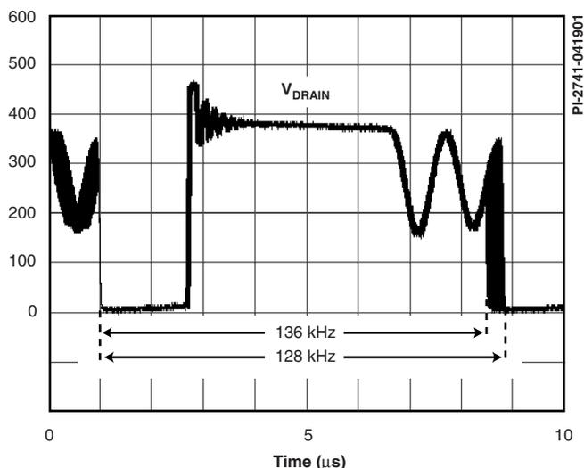
Figure 4. Frequency Jitter.
